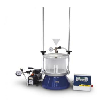
VIBRO-DEAERATOR, electromagnetic, with adjustable vibrating intensity. To vibrate the pyknometer for the evacuation of the air.
