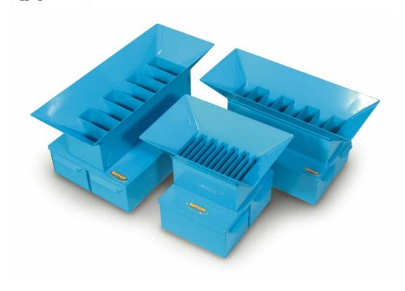
Used for the precise division into two representative portions of materials such as: aggregates, sand, gravel and similar. **Painted steel made**, they are **supplied with** two collecting pans. Multiple models available:
