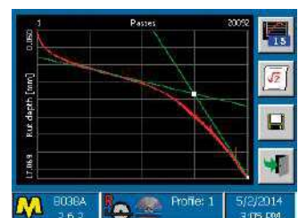
Real time results plot of the rut depth along with the no. of passes.
